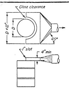
Q = 100 cfm/sq ft barrel top min Duct velocity = 3500 minimum Entry loss = 0.25 VP + 1.78 slot V Manual loading.
