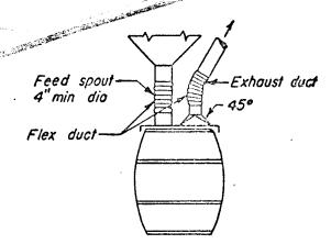
Q = 50 cfm × drum dia (ft) for weighted lid 150 cfm × drum dia (ft) for loose lid Duct velocity = 3500 fpm minimum Entry loss = 0.25 VP
