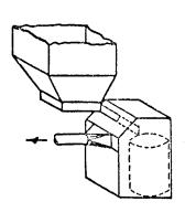
Q=150 cfm/sq ft open face area Duct velocity = 3500 fpm minimum Entry loss = 0.25 VP for 45° toper
