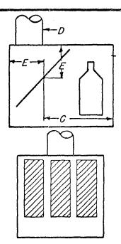
2. Angular Baffle E=D+6" Baffle area = 0.40 WH
