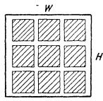
I. Split Baffle or Filters B = 0.75 D Baffle or filter orea = 0.75 WH Filter combustibility Class 2 or better. Consult NBFU or insurance underwriters
