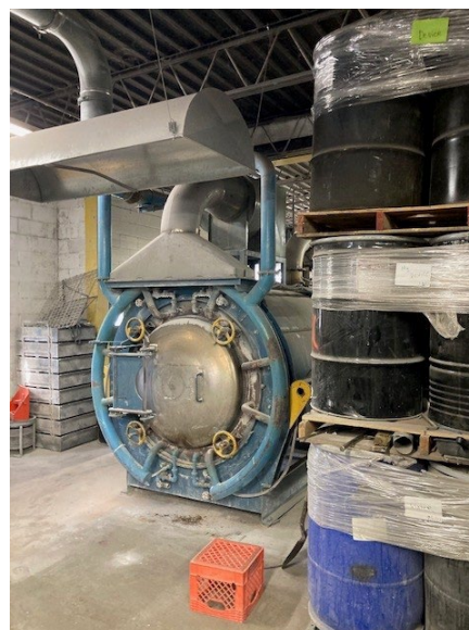
Figure A6. Front of the retort where metal trays containing mercury dust are placed. Photo by NIOSH.
