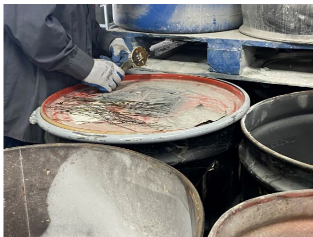
Figure A8. Removing the metal housing for mercury-containing lightbulbs in the disassembly area. Photo by NIOSH.
