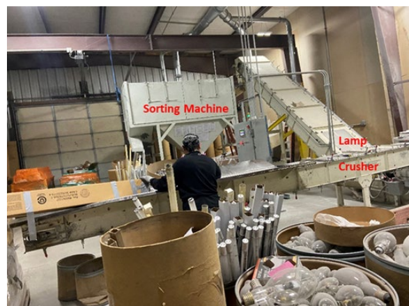
Figure A1. Lamp room conveyor, lamp crusher, and sorting machine. Photo by NIOSH.
