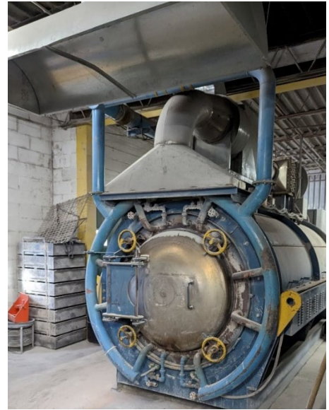
Figure B5. Two overhead exhaust hoods over the cylindrical retort furnace. Photo by NIOSH.
