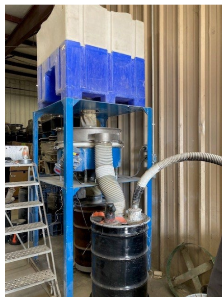
Figure A4. Shaker is designed to separate mercury-containing dusts from fine glass. Photo by NIOSH.
