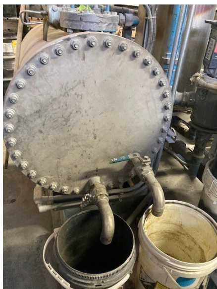
Figure A7. End of the retort where liquid mercury exits through ports into two buckets. Photo by NIOSH.
