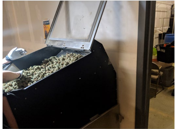
Figure B3. An employee operating the trimming machine with the lid opened while the machine is operating. Photo by NIOSH.
