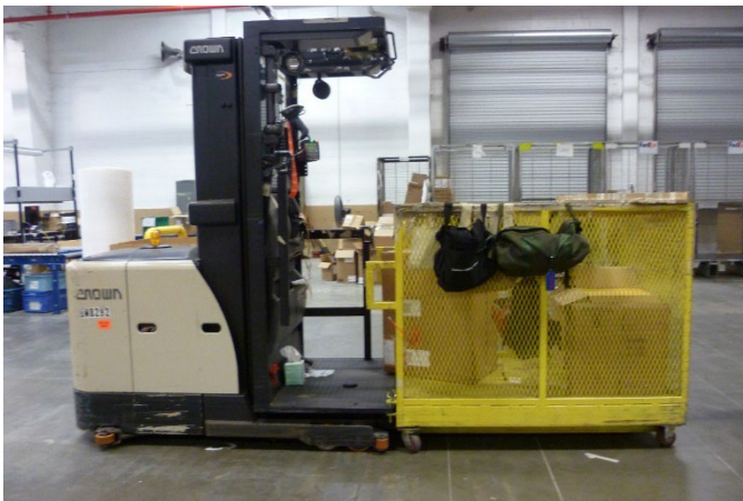
Figure B6. Stock selector used to pick and stow items. Photo by NIOSH.
