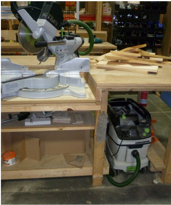
Figure B2. Compound miter saw connected to a mobile dust extractor. Photo by NIOSH.
