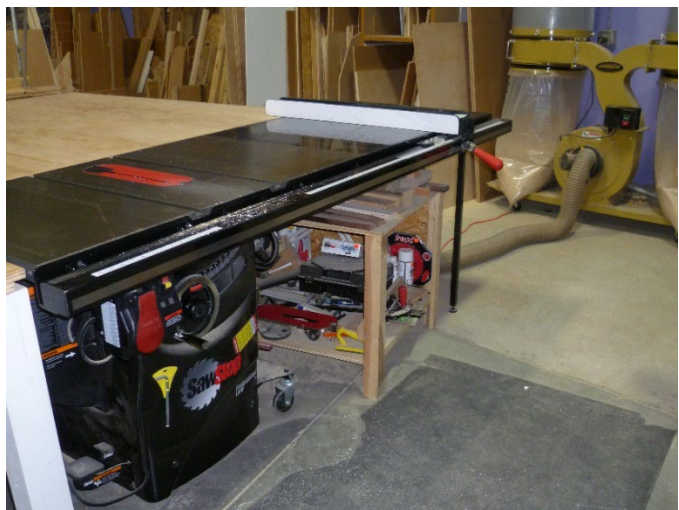
Figure B1. Woodshop table saw with exhaust duct connected to the dust collector. Photo by NIOSH.
