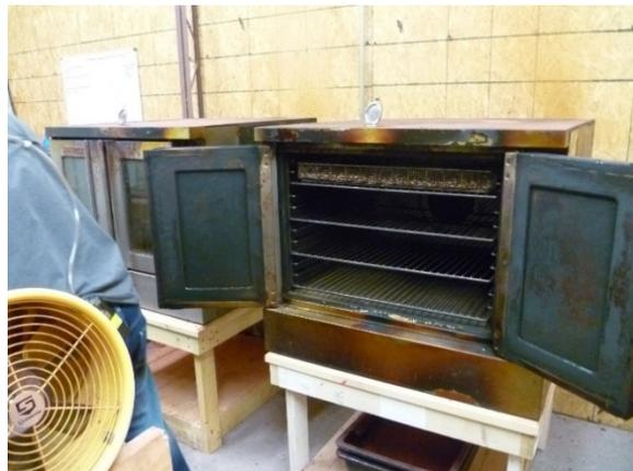
Figure 12. Trays of freshly coated bullets are placed into electrically-heated ovens to harden the paint coating.
