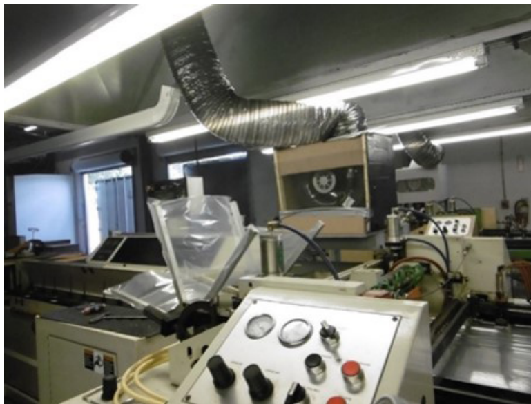
Figure 5. Slot hood local exhaust ventilation on the wicketer. Photo by NIOSH.
