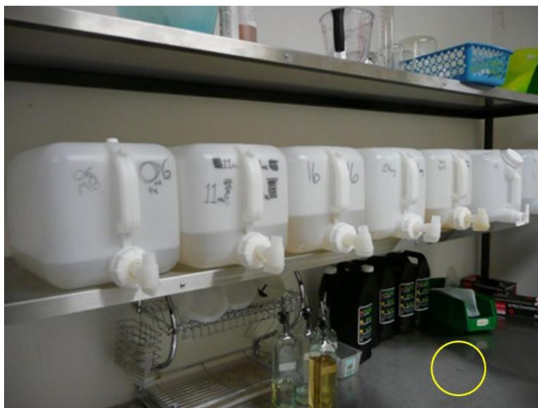
Figure 1. Carboys containing nicotine, propylene glycol, and vegetable glycerin in the back room of a shop. One of the carboys appeared to be leaking, as indicated by fluid on the counter surface below the carboy nozzle and shown inside the yellow circle drawn on the figure. Photo by NIOSH.
