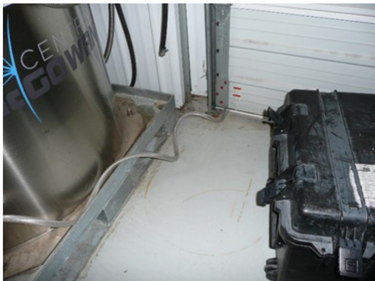
Figure 4. Tubing running from the decarboxylation oven exhaust port to outside the building.
