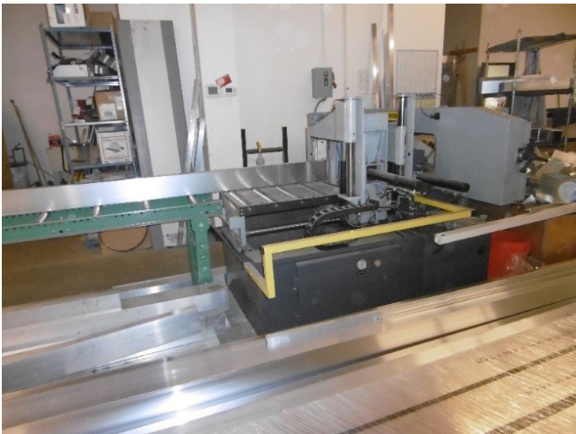
Figure 1. Automated band saw sawing a stick of aluminum alloy. The operating station is to the right of the saw. Photo by NIOSH.
