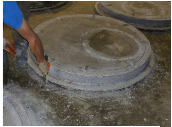
Figure 4. Employee striking the side of the base plate with a claw hammer to remove excess dried concrete. Photo by NIOSH.
