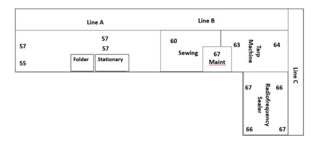
Figure 1. North building CO measurements (ppm) and location during the morning.
