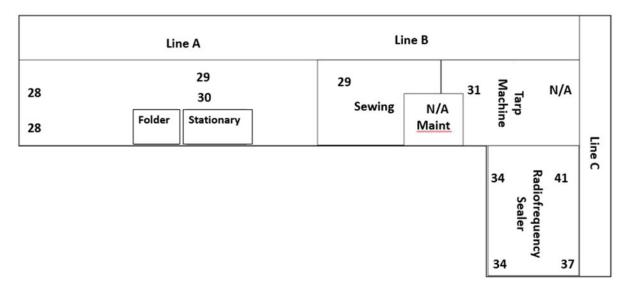
Figure 2. North building CO measurements (ppm) and location during the afternoon.
