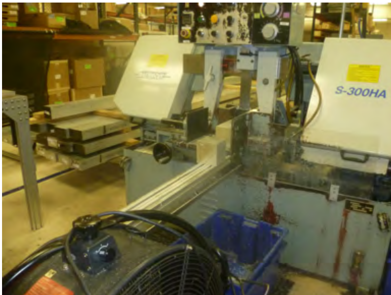
Figure 3. Stock metal cutting machine. Photo by NIOSH.
