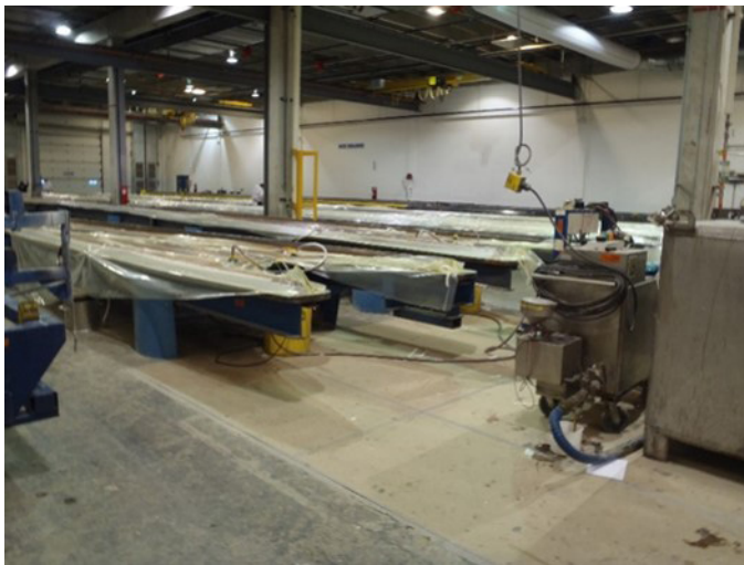
Figure 4. Several web molds during resin infusion. Photo by NIOSH.
