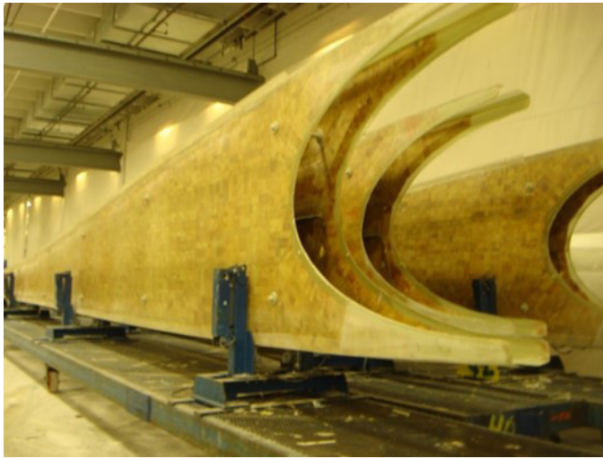
Figure 5. Three webs on storage racks awaiting transfer to Building 1. Photo by NIOSH.
