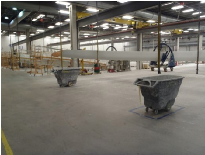
Figure 2. A blade ready for finish coating and final assembly. Photo by NIOSH.
