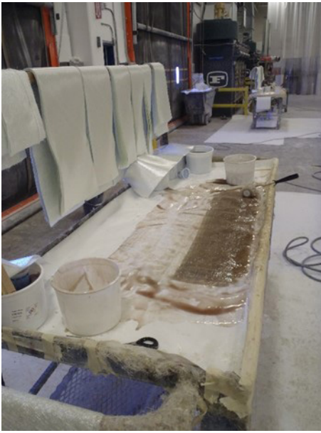
Figure 1. A resin-impregnated fiberglass patch, ready to be applied to either the interior or exterior blade seam. Photo by NIOSH.
