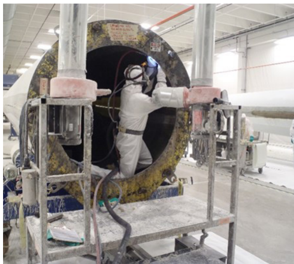
Figure 11. Employee wearing a supplied air respirator performing inside blade cut and trim work using a grinder equipped with local exhaust ventilation. Photo by NIOSH.
