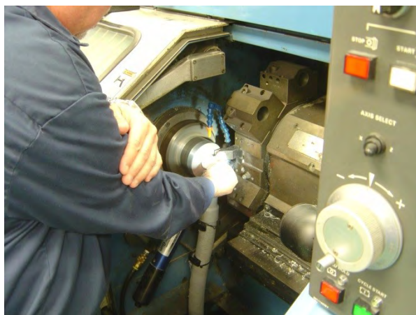
Figure 7. Plastic patella lathe. Photo by NIOSH.
