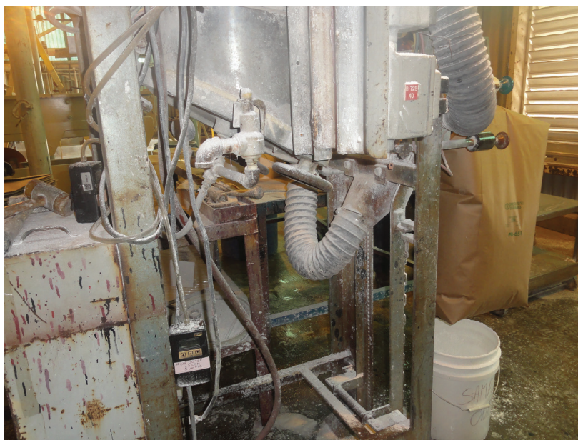
Figure 2. Excess duct work caused dust to accumulate in the duct. Photo by NIOSH.
