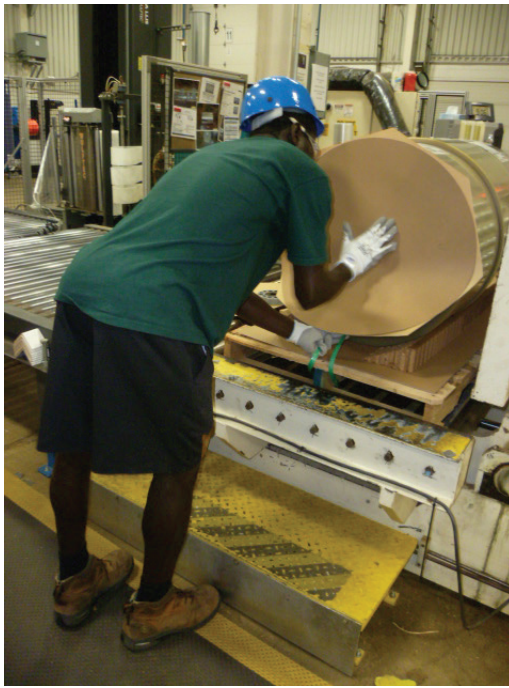
Figure 3. Employee installing a strap to hold a paper roll on the pallet. Photo by NIOSH.
