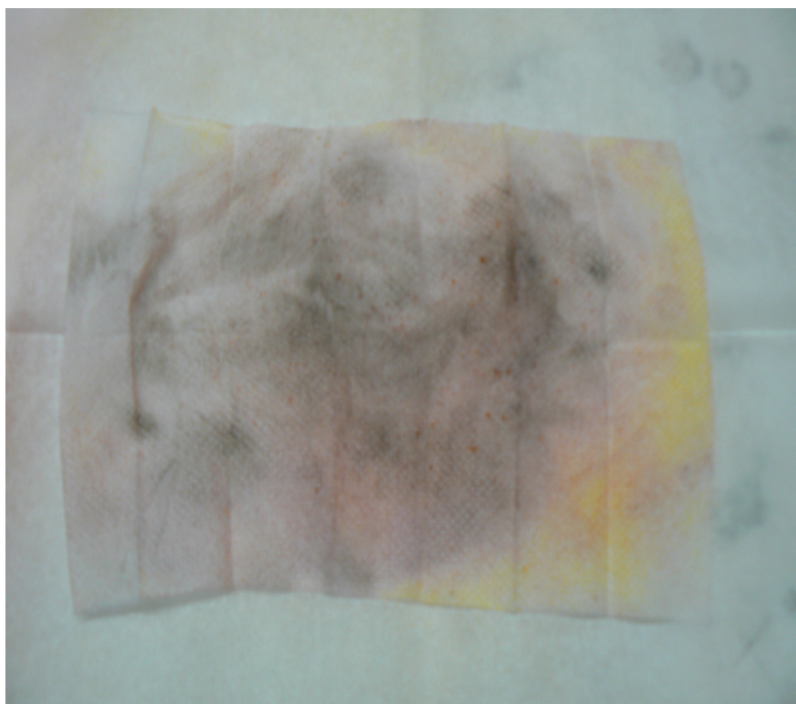
Figure 1. A wipe taken from employee's hands turned red, indicating the presence of lead.
