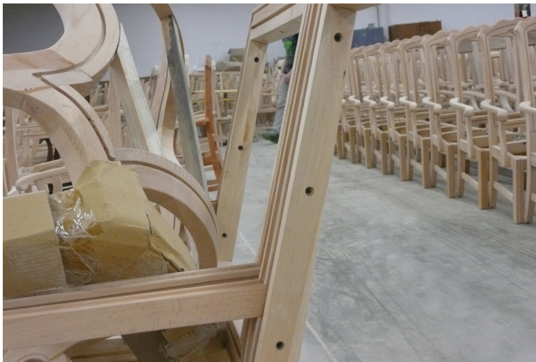
Figure 2. Screw holes in chair frames that were to be filled with epoxy resin. Photo by NIOSH.
