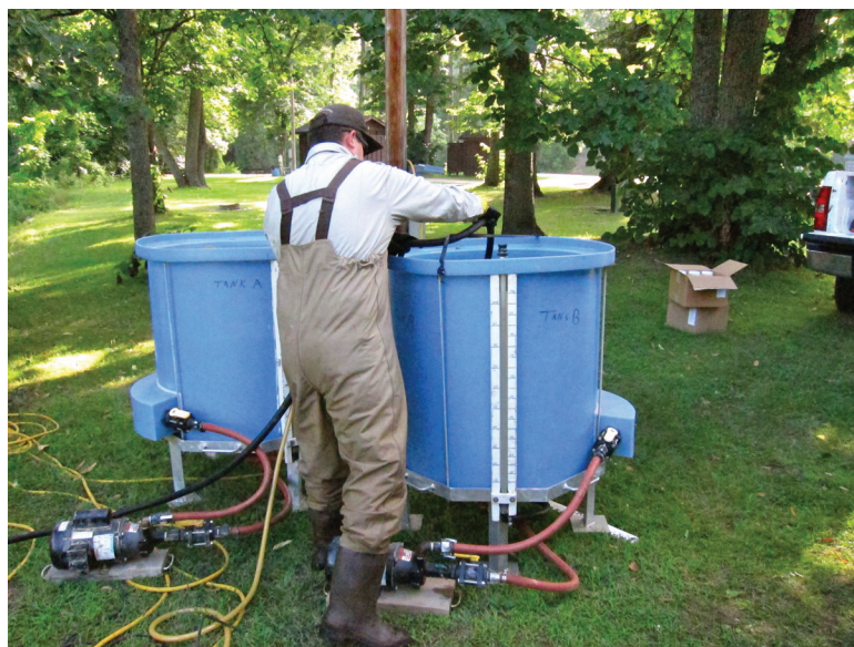
Figure 2. Manual pouring of the Bayluscide wettable powder pesticide into two large vats before it is pumped into a river. Photo by NIOSH.
