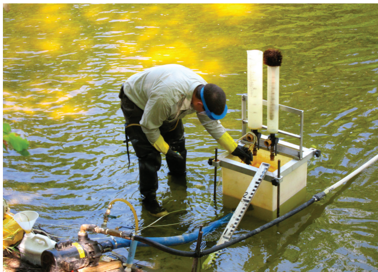
Figure 1. Manual application of the TFM liquid pesticide in a river at low flow rates. Photo by NIOSH.
