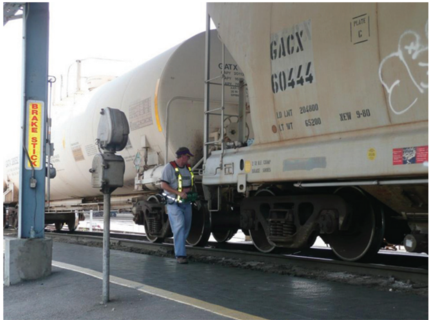
Figure 1. Freight conductor using the RCL device to direct rail cars up the hump to be released and sorted by gravity.
