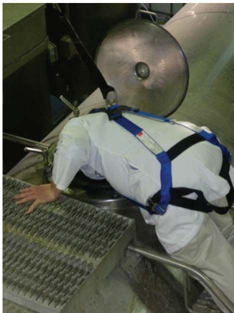
Figure 1. Equipment inspector partially enters a milk tanker while wearing a full-body harness provided by the plant.
