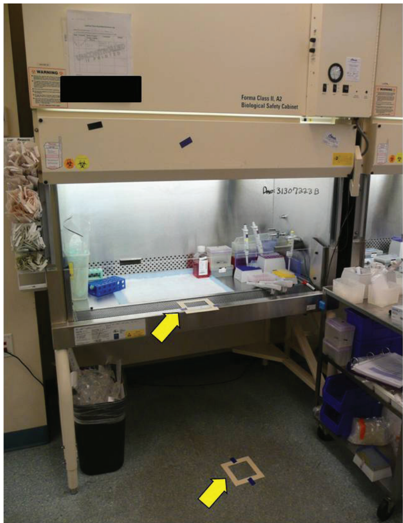
Figure 2. A BSC containing a sample template on the airfoil of the BSC and a sample template on the floor directly in front of the BSC.
