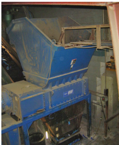
Figure 3. Grinder used for recycling plastic drums.
