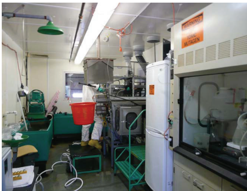
Figure 2. Photograph of the injection room, with fume hood on the right, an employee operating the automated injection machine in the center, and bisazir storage refrigerator between them. Sea lampreys are held in the tank on the left before sterilization.
