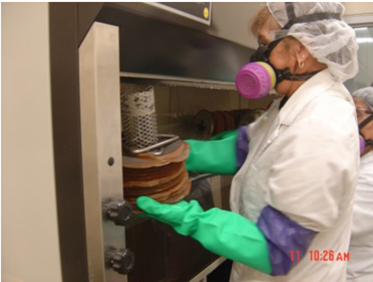
Figure B2. An employee preparing to submerge a spindle of egg rings into the formaldehyde tank located in a lab fume hood. Photo by NIOSH.
