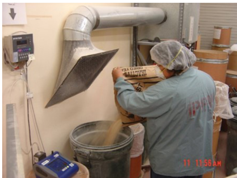
Figure 2. Scale and LEV hood for insect diet ingredient preparation. Photo by NIOSH.
