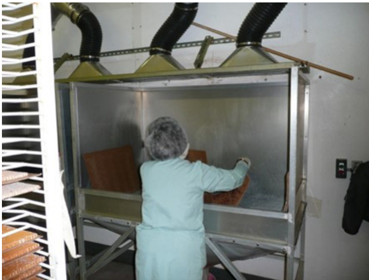
Figure 3. An employee standing at the face of the work booth performing the Hexcel stripping operation in the booth. Photo by NIOSH.
