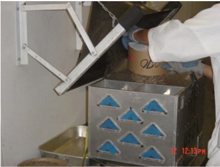
Figure 5. An employee manually dumping irradiated moths from cylindrical containers into the shipping crate. Photo by NIOSH.
