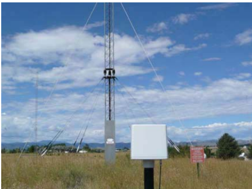
Figure 3. HF radio station antennas (background) with RF meter in the foreground.
