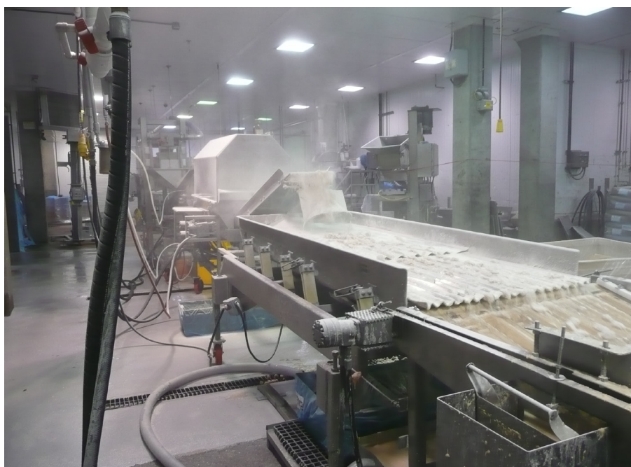
Figure 6. Unenclosed conveyor belt without local exhaust ventilation and transfer point between machines.
