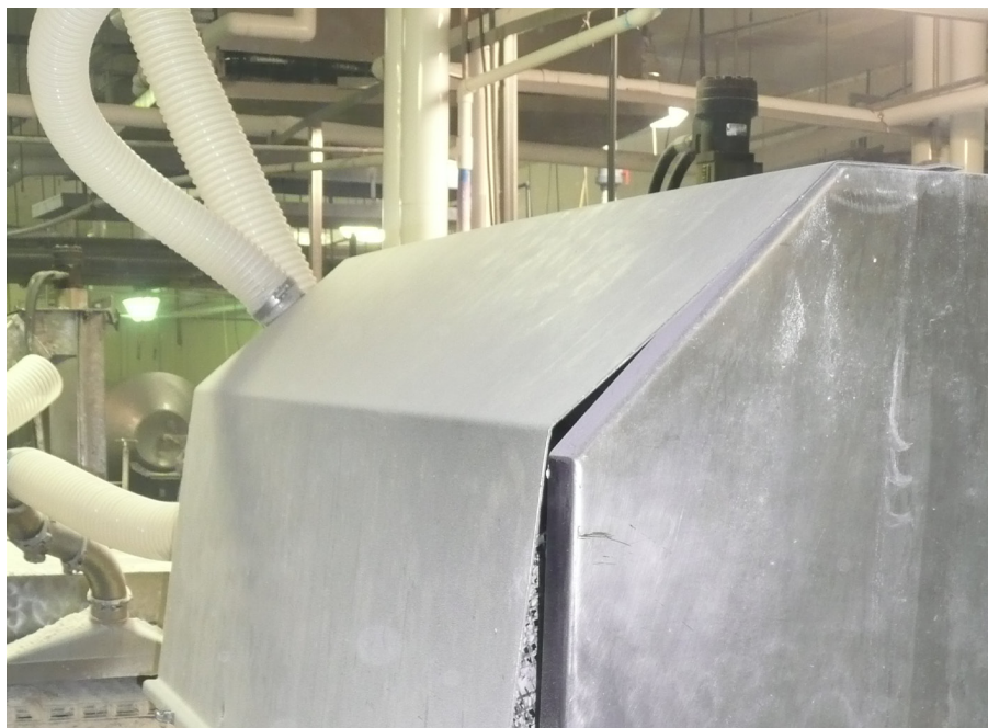
Figure 7. Open enclosure on breasting machine.
