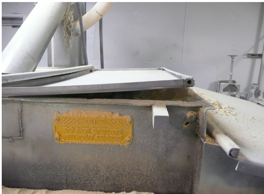
Figure 5. Dispensing hopper lid on breeding machine.
