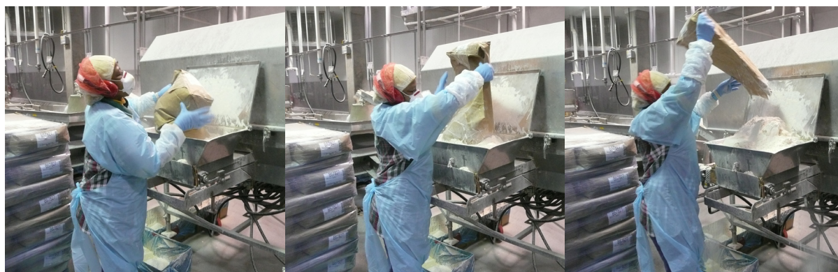
Figure 8. Employee transferring dry powdered ingredients into a breasting machine hopper at breathing zone height.
