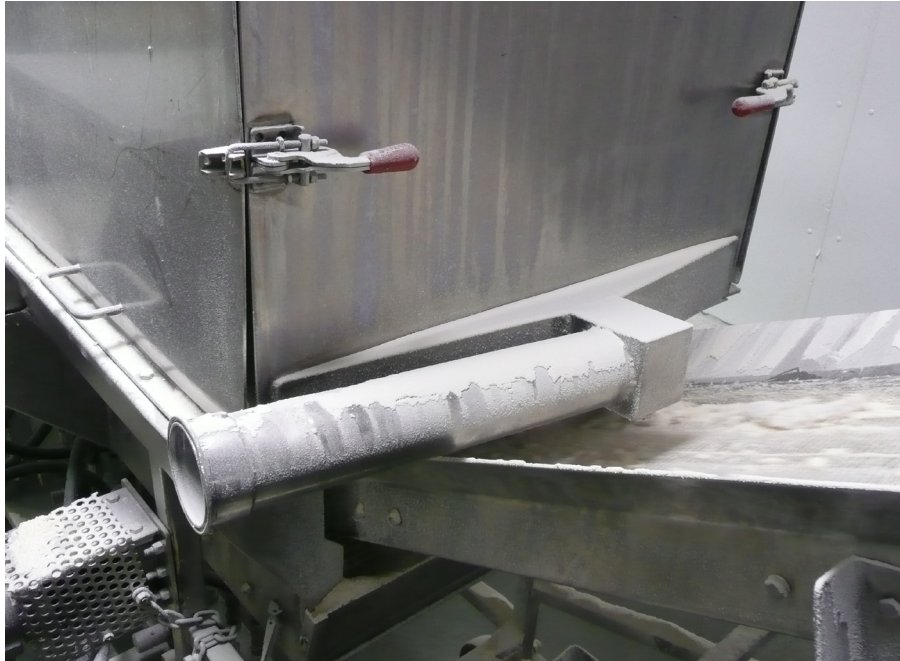
Figure 3. Local exhaust ventilation attachment not in use on breeder.
