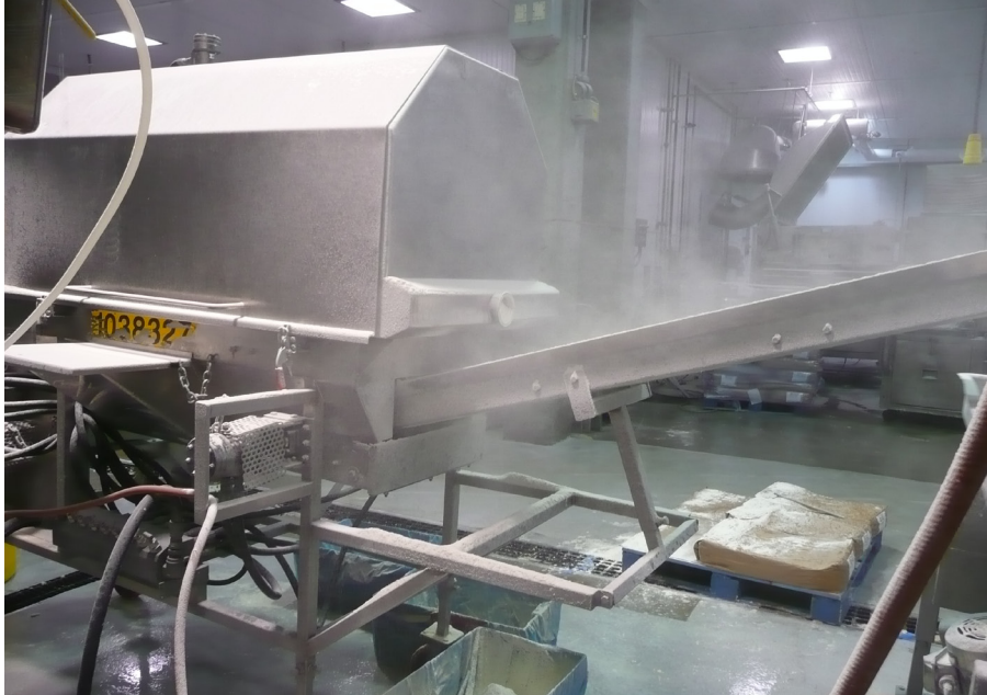
Figure 4. Local exhaust ventilation attachment not in use on breeder and non-enclosed product conveyer belt.
