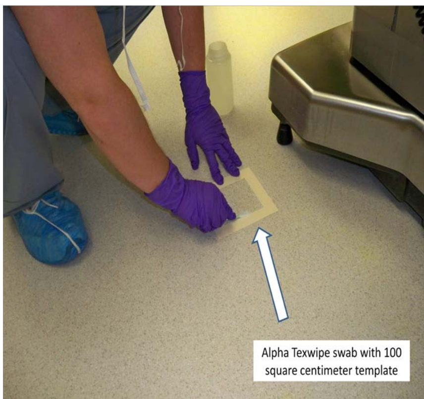
Figure 4. Collection of wipe sample with Alpha Texwipe swabs with a 100 cm 2 template.
