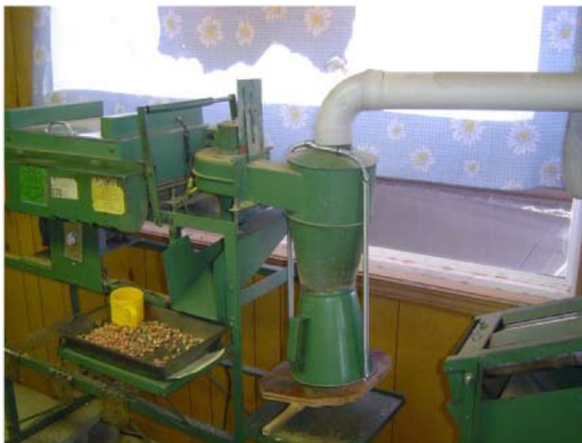
Figure 1. Peanut grading machine with retrofitted exhaust ventilation duct in 2008
