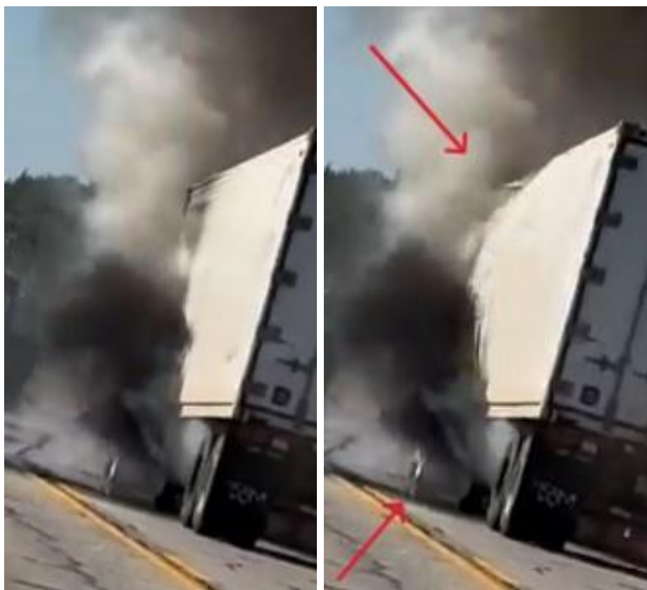
Photo 7 and Photo 8. Driver side of trailer just prior to explosion (left photo) and change of smoke behavior and expansion of container as explosion is occurring (right photo). (Photos courtesy of fire department)
