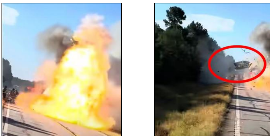
Photo 26 and Photo 27. These images provide a sense of the amount of energy released by the explosion in terms of a blast, projectiles, and thermal radiation. The image on the right shows the latched door that was blown off the trailer.
