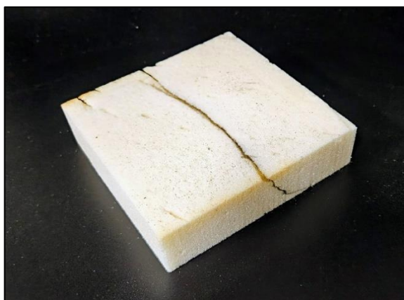
Photo 15 and Photo 16. One of the foam samples prepared for testing in the cone calorimeter (left photo) and amount of flame generated by the foam sample during a cone calorimeter test (right photo).
