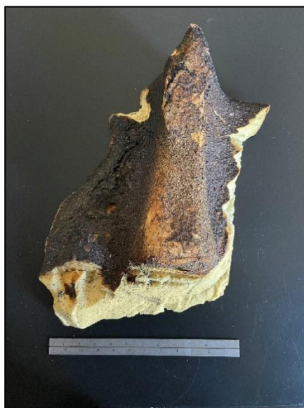
Photo 13 and Photo 14. The foam sample from the trailer flooring section that was provided for testing. Bottom of the sample (left photo) and top of the sample (right photo).
