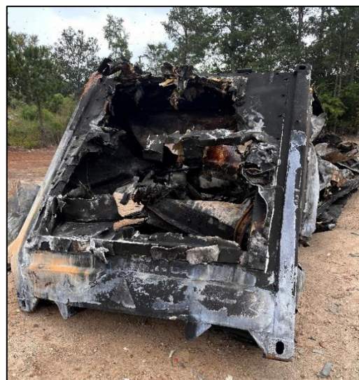
Photo 9 and Photo 10. Photographs of the remains of the refrigerated trailer. Rear view on the left and front view on the right. Most of the foam insulation had been burned out of the front portion of the trailer. (Photos courtesy of UL FSRI)
