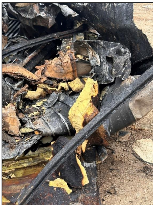
Photo 11 and Photo 12. Some of the remaining foam insulation. Partially charred foam from a wall panel (left photo) and partially charred foam in the floor section of the trailer (right photo).
