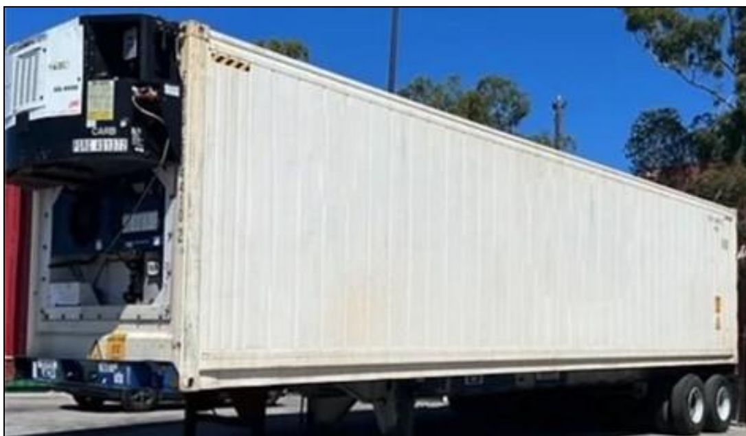
Photo 2. Type 111 Intermodal Freight Container secured to trailer chassis with genset. (Photo courtesy of UL FSRI)
