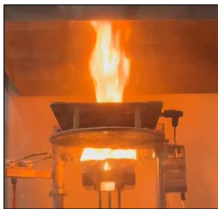
Photo 15 and Photo 16. One of the foam samples prepared for testing in the cone calorimeter (left photo) and amount of flame generated by the foam sample during a cone calorimeter test (right photo).
