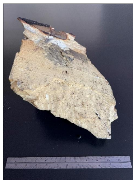
Photo 13 and Photo 14. The foam sample from the trailer flooring section that was provided for testing. Bottom of the sample (left photo) and top of the sample (right photo).
