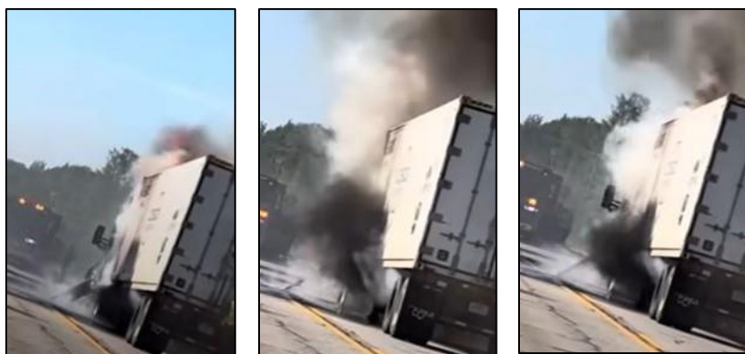
Photo 23, Photo 24, and Photo 25. These images are one second apart between 0932 and 0933. Dense black smoke flow from under the trailer once again is pushing out. This was seconds before the explosion.
