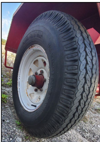
Photo 3: Passenger side tire with visible size, type and capacity rating. Wheel displays rusting and flaking. (Photo by NIOSH)
