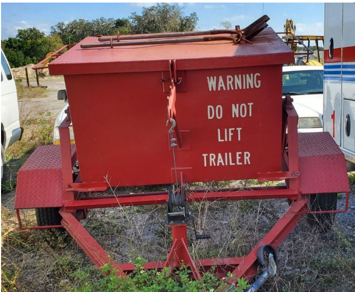
Photo 1: Front of sand trailer with front stabilizing jack in retracted position located on the front frame behind the trailer coupler (not visible), while being stored at the city's storage yard. (Photo by NIOSH)
