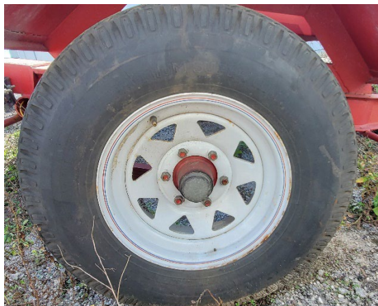
Photo 4: Driver side tire showing extensive weathering of the tire and rusting and flaking of the wheel. (Photo by NIOSH)
