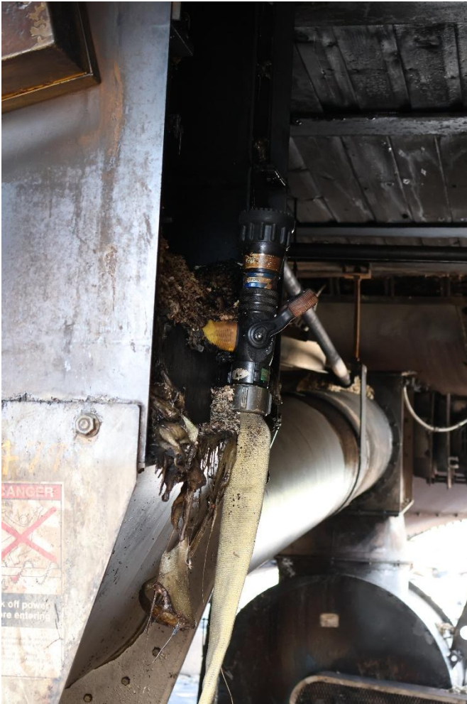
Image 7 and 8. View of nozzle in chute (left) and 3 ft diameter hole into base of silo (right), post-incident. (Sources: State Fire Marshal's Office and NIOSH)
