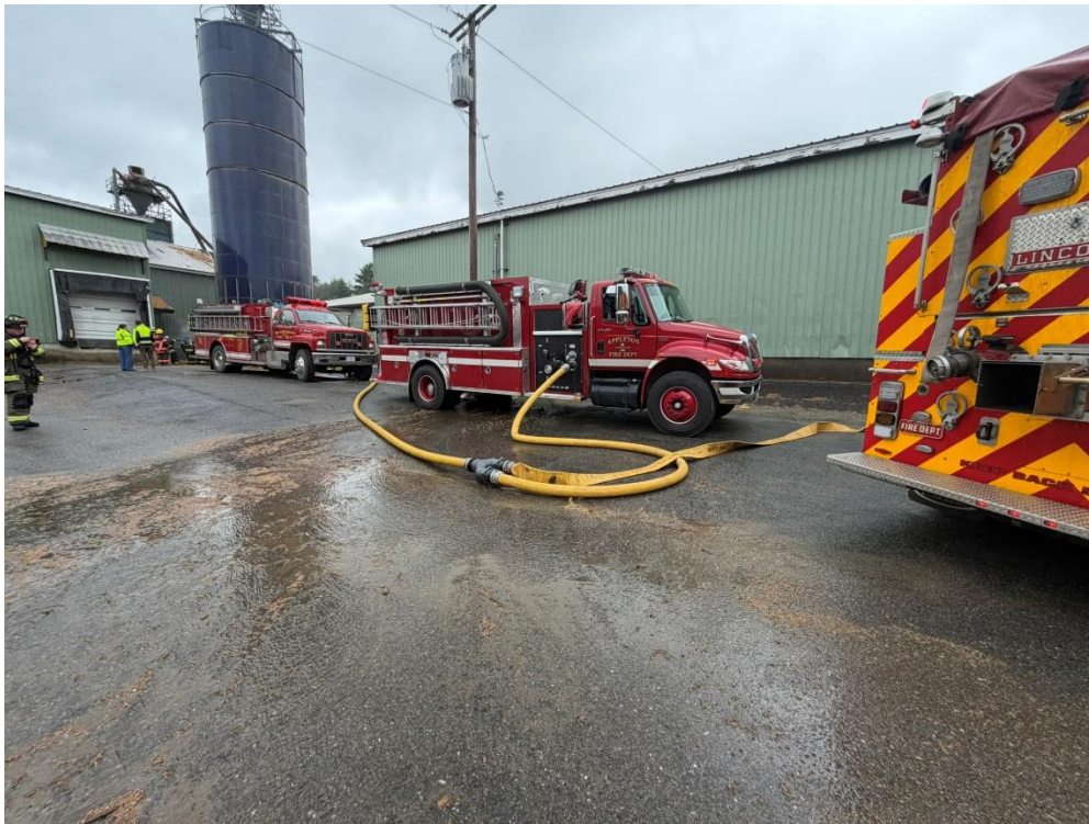
Image 10. View of apparatus placement near incident silo with Engine 70-1 supplying Engine 40-2. (Source: Fire department)
