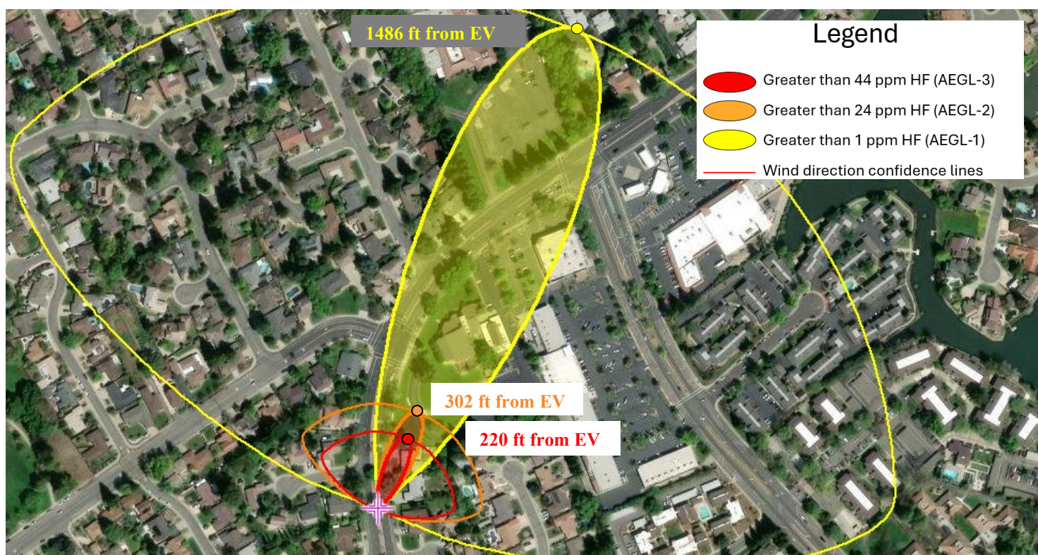
Figure 6. MARPLOT Map of AEGL [60 min] Threat Zones (100% Battery Involvement Assumption)
