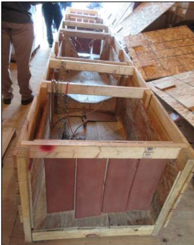
Photo 1: Tunnel Prop made from a ladder shipping box (Photo by NIOSH)
