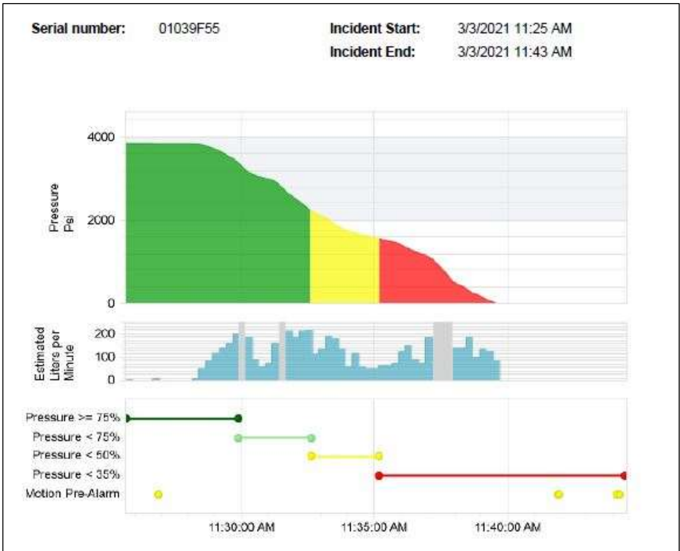
Graph D: Fourth cylinder on March 3, 2021. Used for second opportunity for culvert tube drill. (Graph by SCBA manufacturer)
