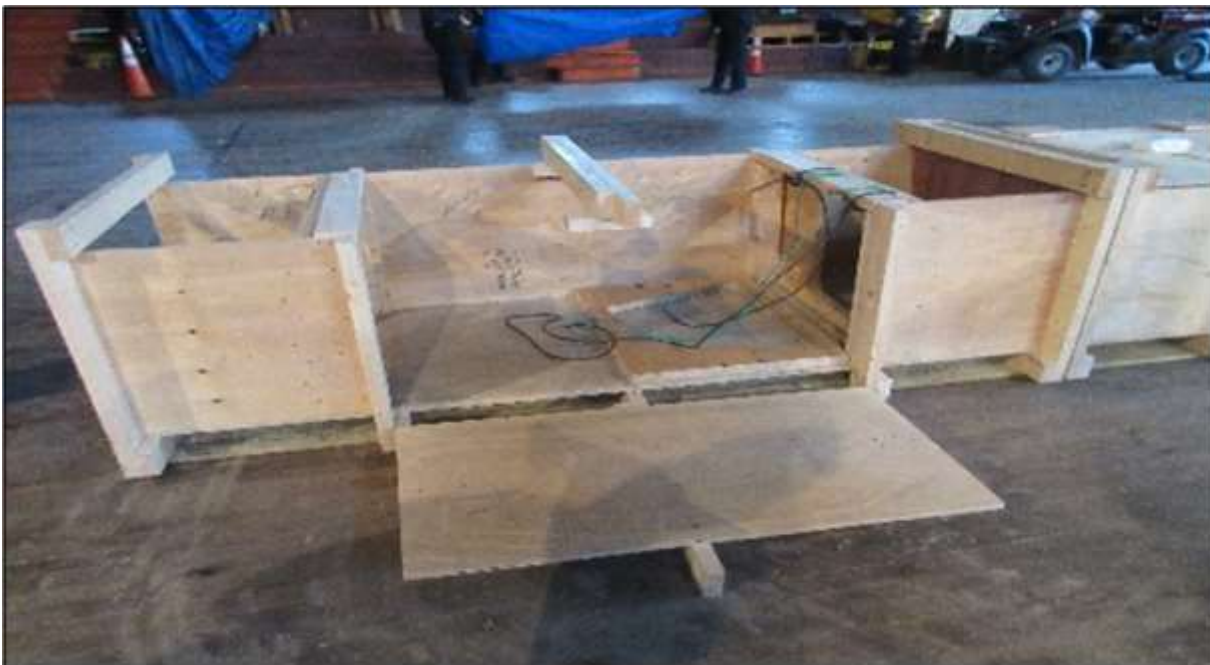
Photo 4: New tunnel prop with side collapsed (Photo by NIOSH)
