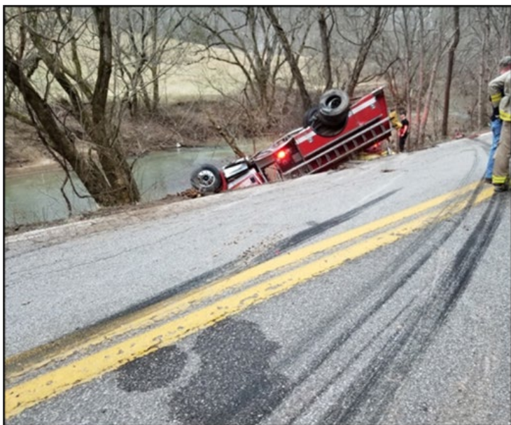
Overturned Engine 22 with tire skid marks on the roadway where the driver lost control of the engine. (Photo courtesy of the Fire Department)
