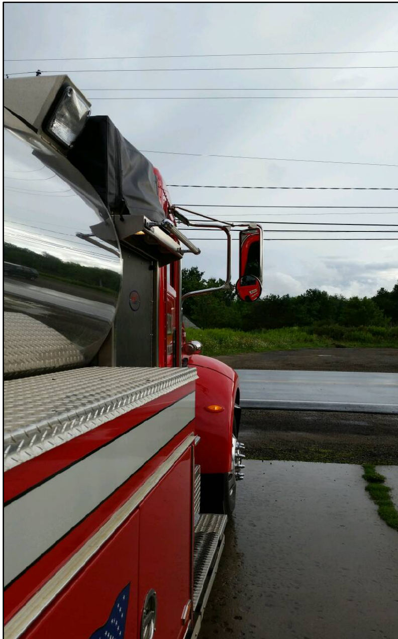
Photo 2. Photo of the passenger side mirror on Tanker 72. Photo shows the narrow field of view that the right-side mirror provides. (NIOSH photo)
