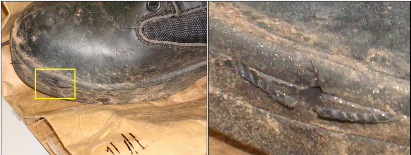
Photo 7 (left) and Photo 8 (right – enlarged). Right boot worn by victim. Note hole near toe – probable exit hole where current exited body. This area of boot corresponds with burn injuries identified in coroner’s report. (NIOSH photos.)
