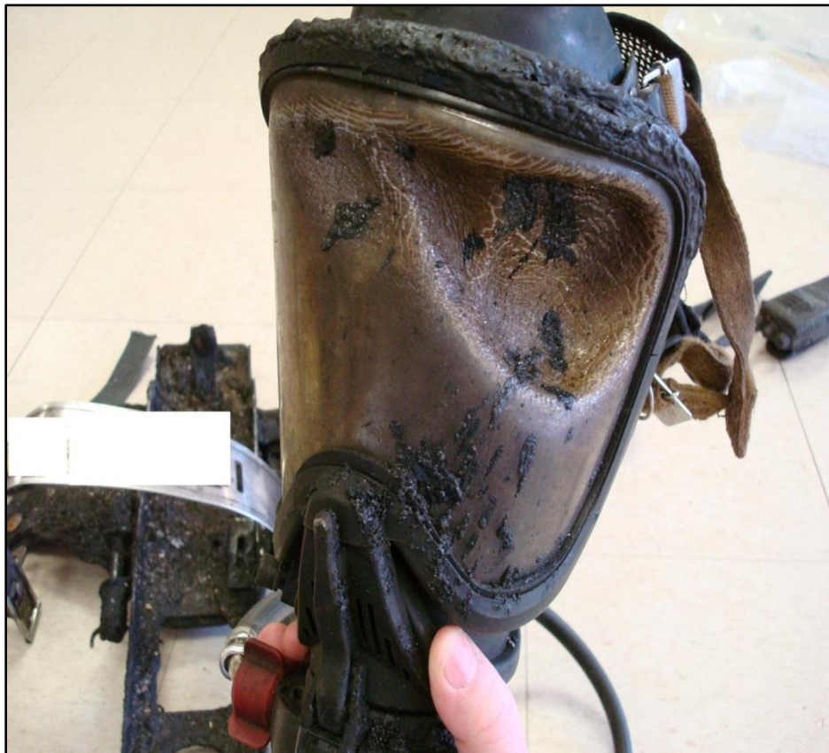
Photo 1. Victim's facepiece showing thermal degradation. (NIOSH Photo.)
