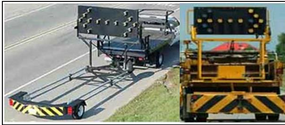
Photos 4(left) and 5(right) show examples of truck mounted attenuators.
