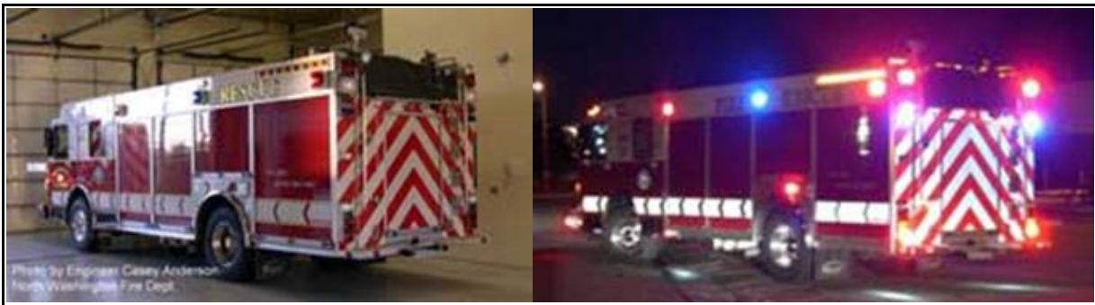
Photos 8(left) and 9(right) show reflective directional arrow markings in daylight and darkness. (Photo courtesy of North Washington Fire Protection District, Denver, CO).
