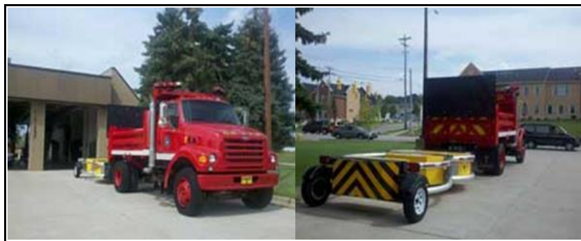
Photos 6(left) and 7(right) show a surplus municipal dump truck that was converted into a truck mounted attenuator.
