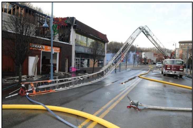
The collapsed aerial ladder (Courtesy of Fire Department)
