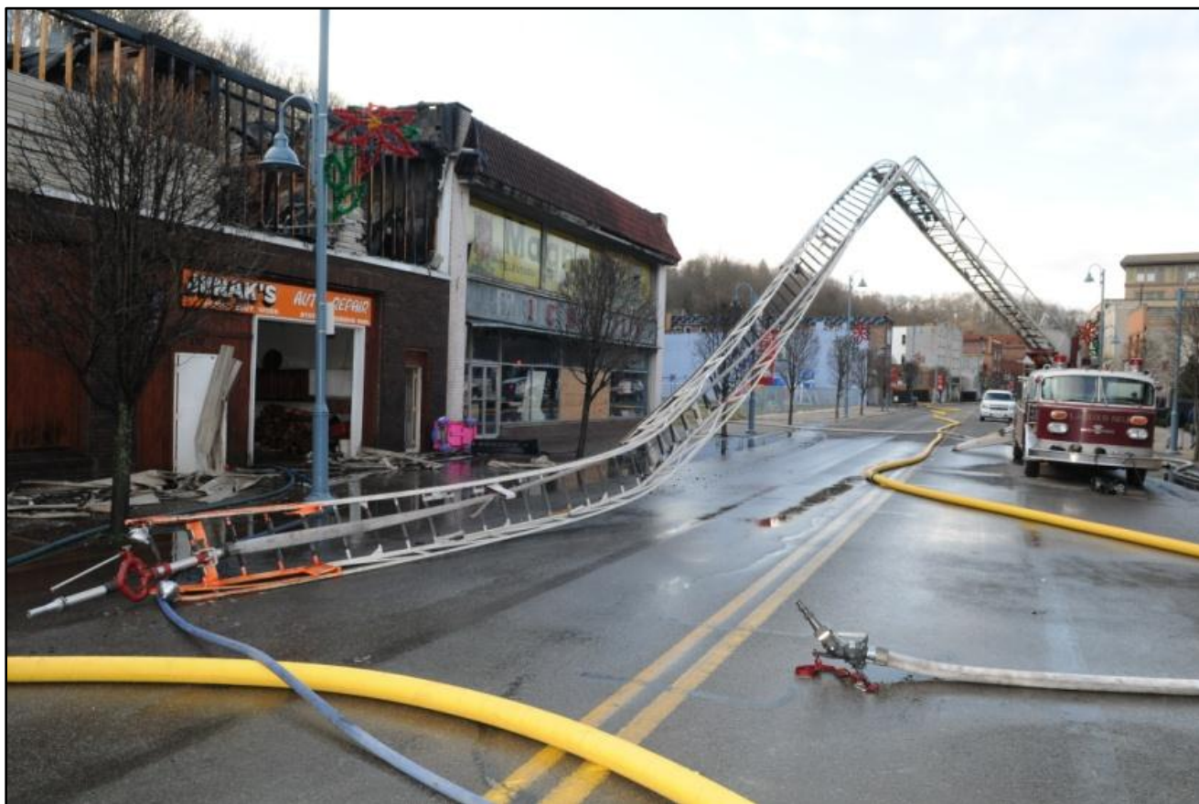
Photo 5. Note 5-inch supply hose laid from one side of the street to the other causing the driver of the aerial apparatus to stop short of fire structure. (NIOSH Photo)
