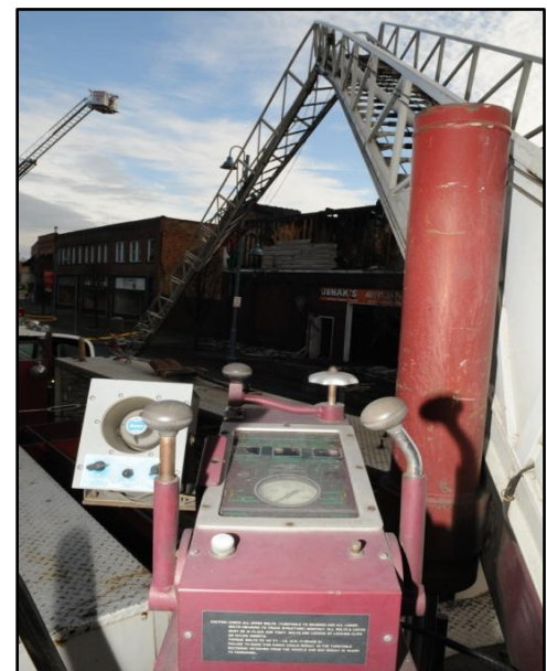
Photo 3. Aerial ladder control pedestal (Courtesy of the Fire Department)
