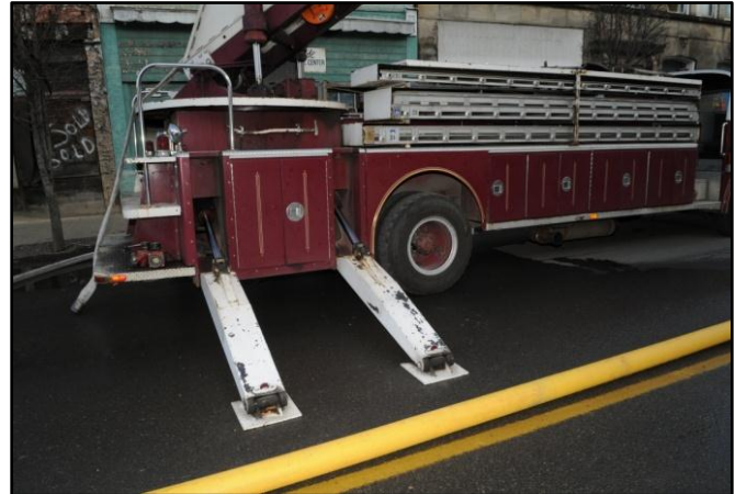
Photo 2. Shows the two sets of hydraulic outriggers. (Courtesy of the Fire Department)
