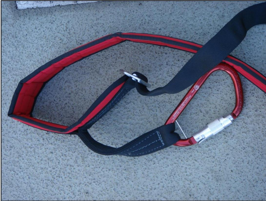
**Photo 1. Identical type of ladder safety belt worn by the victim and other fire personnel when climbing the ladder.**
