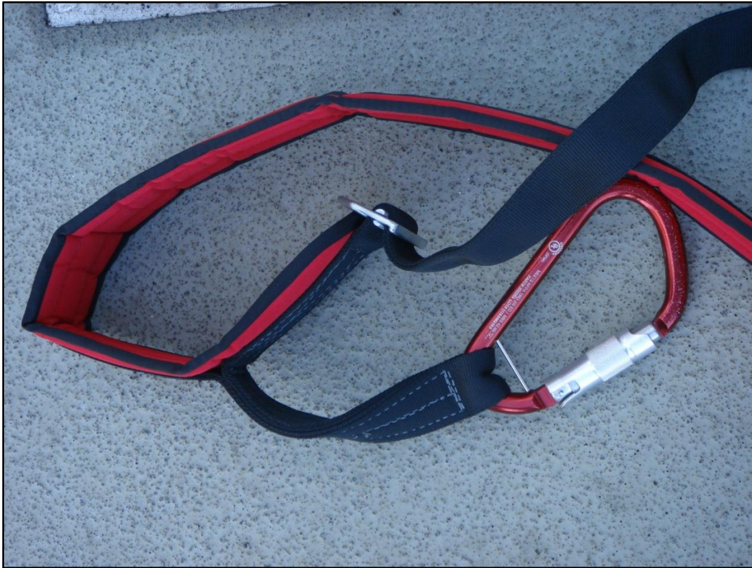
Photo 1. Identical type of ladder safety belt worn by the victim and other fire personnel when climbing the ladder. (NIOSH photo.)
