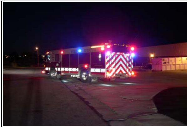
Photos 16(left) and 17(right) show reflective directional arrow markings in daylight and darkness.
