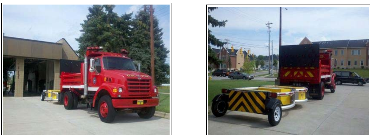
Photos 14(left) and 15(right) show a surplus municipal dump truck that was converted into a truck mounted attenuator. (Photos courtesy of Grand Rapids, MI, Fire Department).
