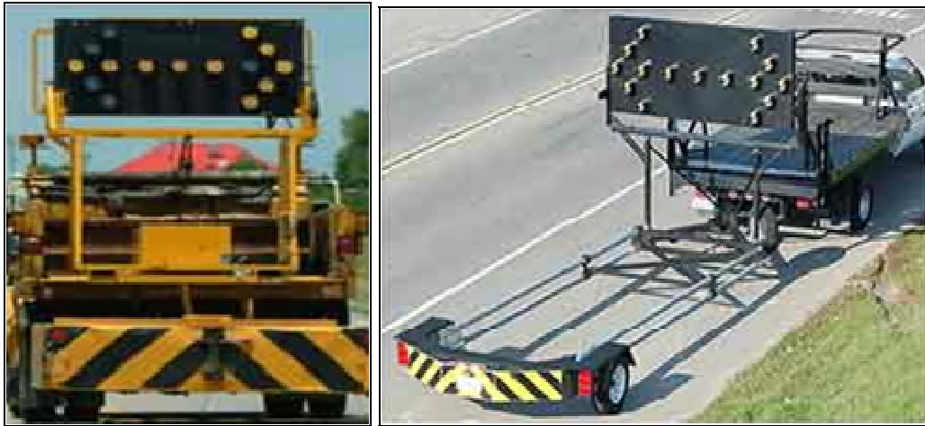
Photos 12(left) and 13(right) show examples of truck mounted attenuators.
