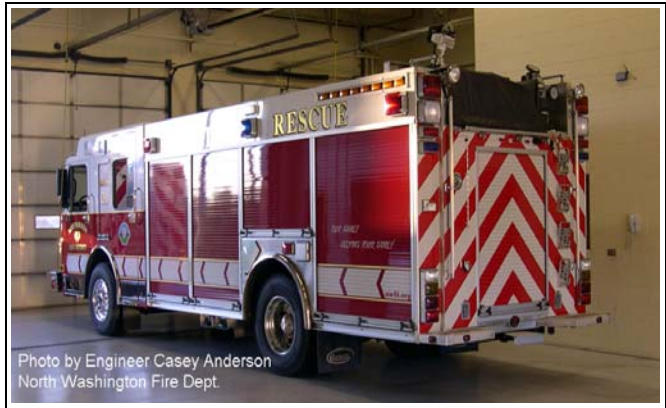
Photos 16(left) and 17(right) show reflective directional arrow markings in daylight and darkness.
