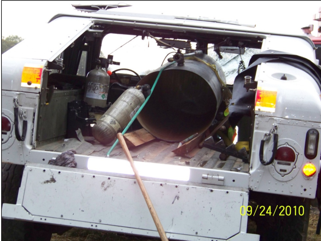
Photo shows a rear view of the Humvee following the explosion. The water tank is seen in the center of the photo. Note that the bottom of the tank has completely separated from the rest of the tank. A motorized hose reel was mounted just in front of the tailgate. (Photo Courtesy of Sheriff's Office)
