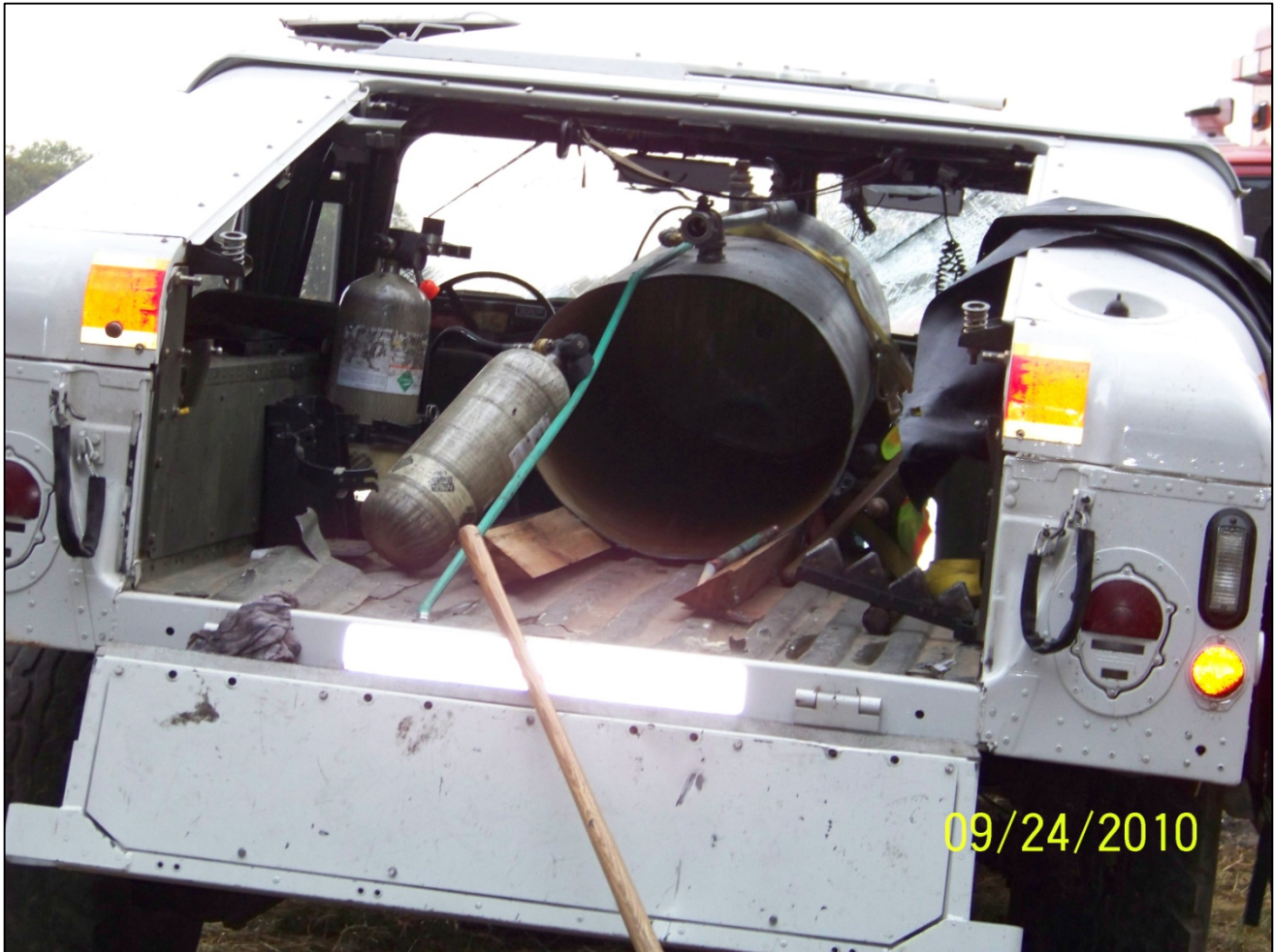
Photo 8. Photo shows remains of the water tank in the bed of the Humvee after the explosion. The bottom of the water tank separated and struck the hose reel, propelling the hose reel over the tailgate. The hose reel is believed to have struck and fatally injured the victim. (Photo courtesy of the Sheriff's Office)
