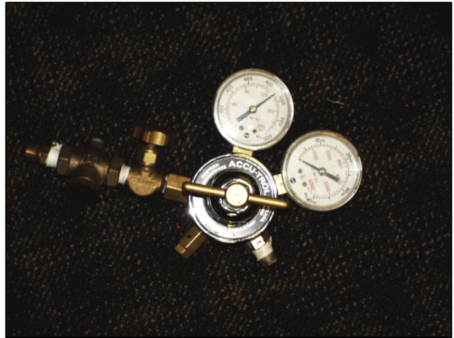
Photo 1 (left) and Photo 2 (right). Photo 1 is the regulator used at the time of the incident. Photo 2 was reported to be the regulator used by the fire department who originally constructed the water delivery system.
