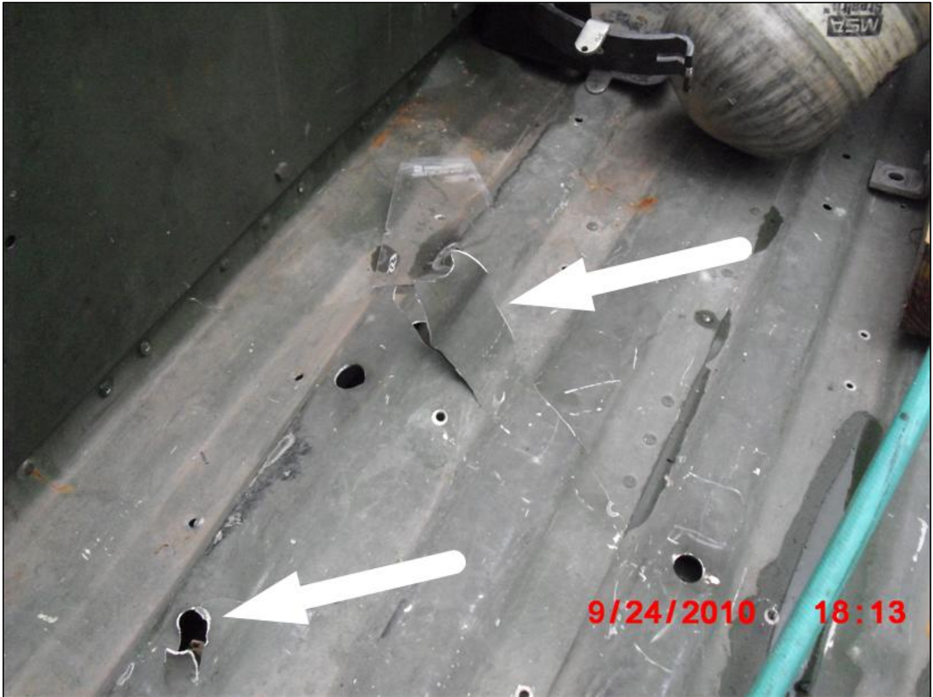
Photo 10. Photo shows the bolt holes through the bed of the Humvee where the motorized hose reel was mounted. The force generated by the end of the exploding tank striking the hose reel ripped the hose reel mounting bolts through the Humvee's bed. Ripped metal at the location of bolt holes indicated by the arrows. (Photo courtesy of the Sheriff's Office)
