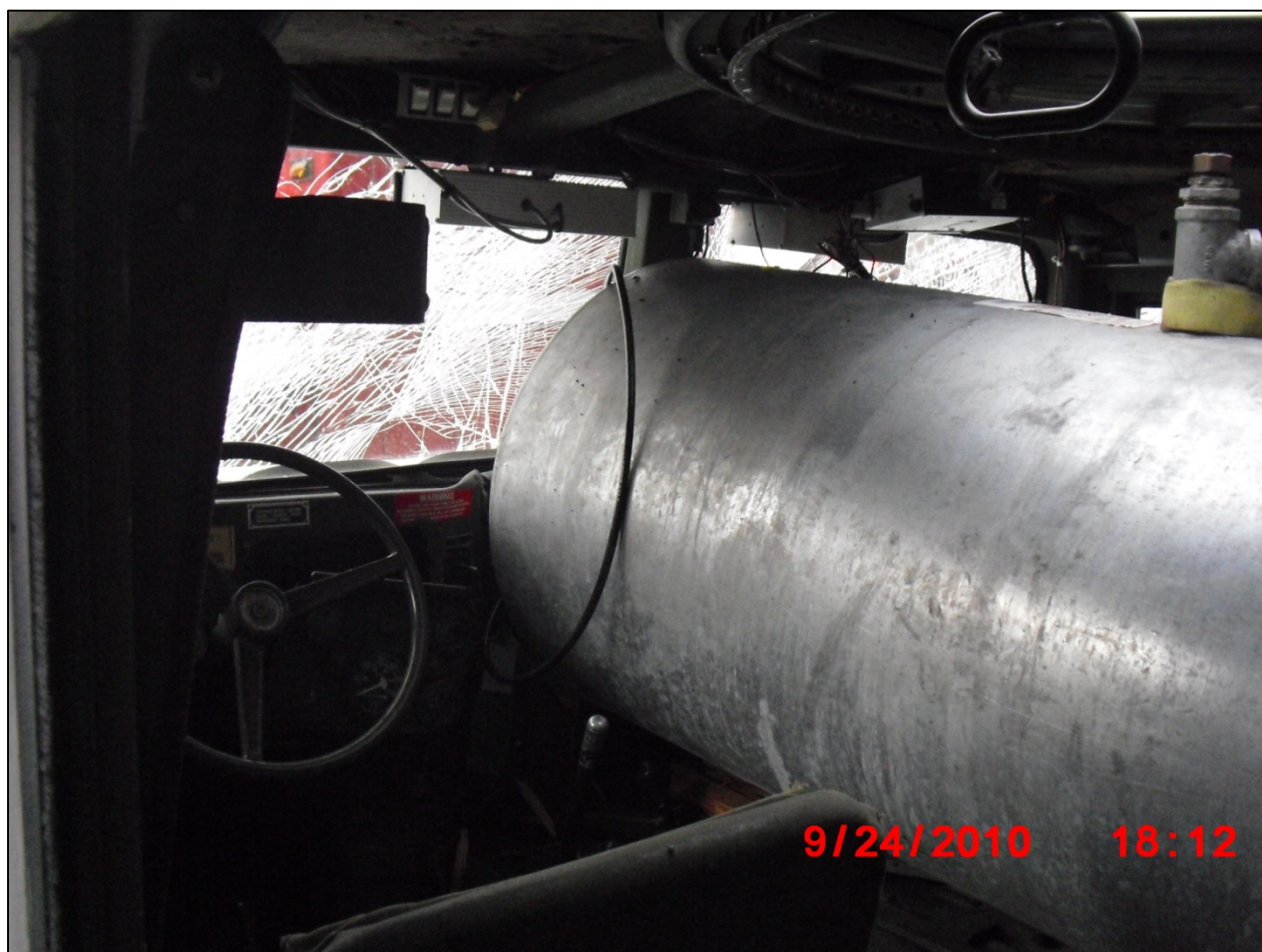
Photo 9. Photo shows how the explosion propelled the front end of the water tank against the Humvee's dashboard. The force of the water tank impacting against the dashboard shattered the windshield.
