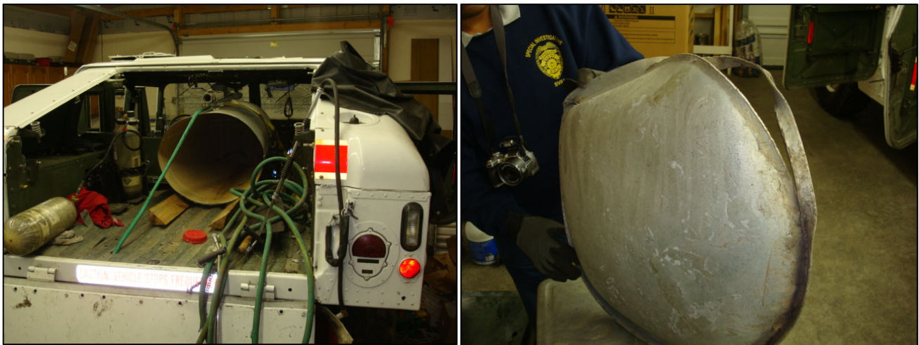
Photo 5 (left) and Photo 6 (right). Photo 5 shows the location of the 120-gallon water tank mounted horizontally in the bed of the Humvee. Note that the tank moved forward after the explosion. Photo 6 shows a close-up of the tank's bottom which separated.
