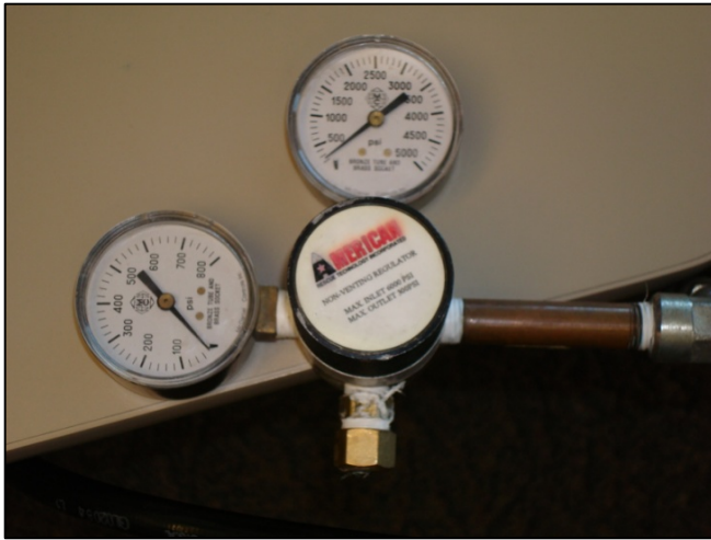
Photo 1 (left) and Photo 2 (right). Photo 1 is the regulator used at the time of the incident. Photo 2 was reported to be the regulator used by the fire department who originally constructed the water delivery system.
