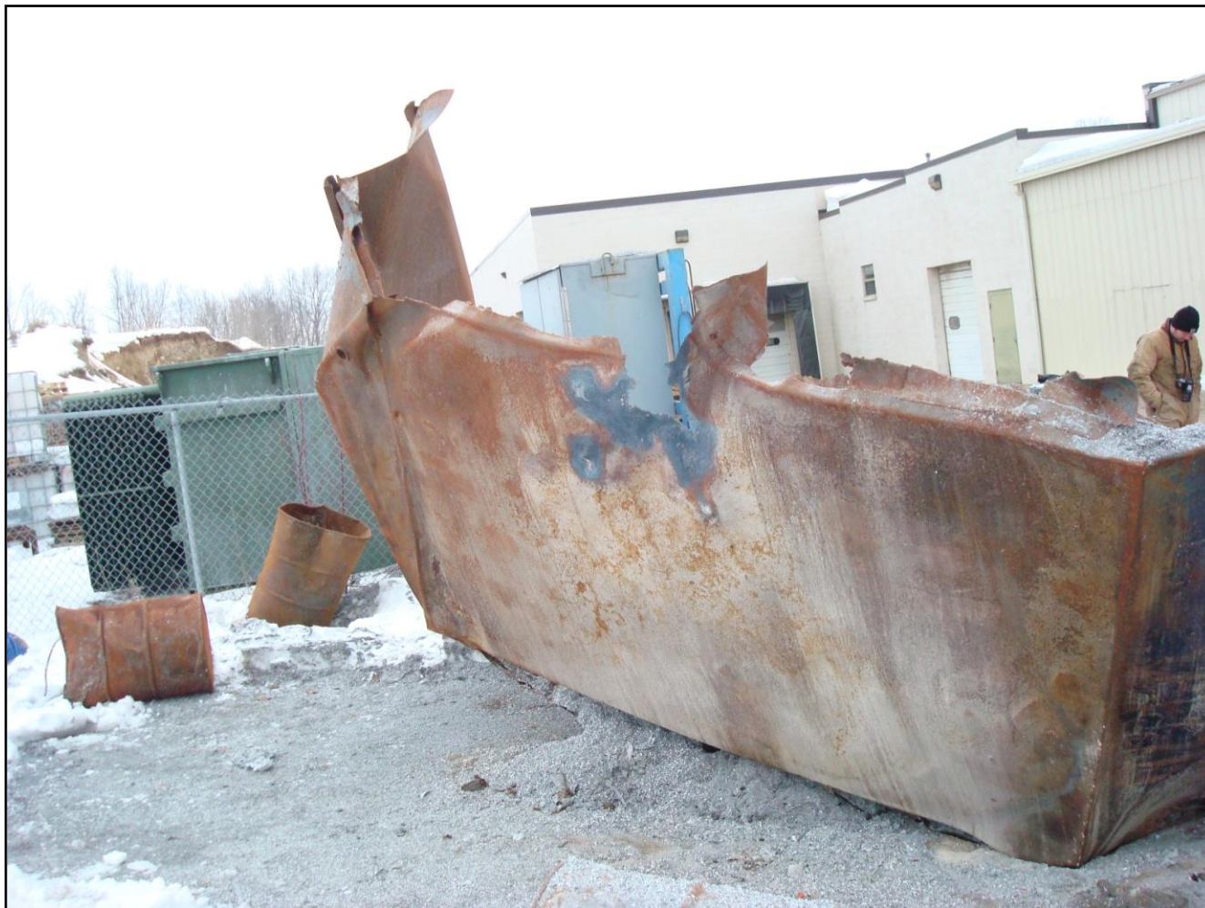
Photo 5. Bottom of the dumpster showing the origin of the fire in the dumpster.
