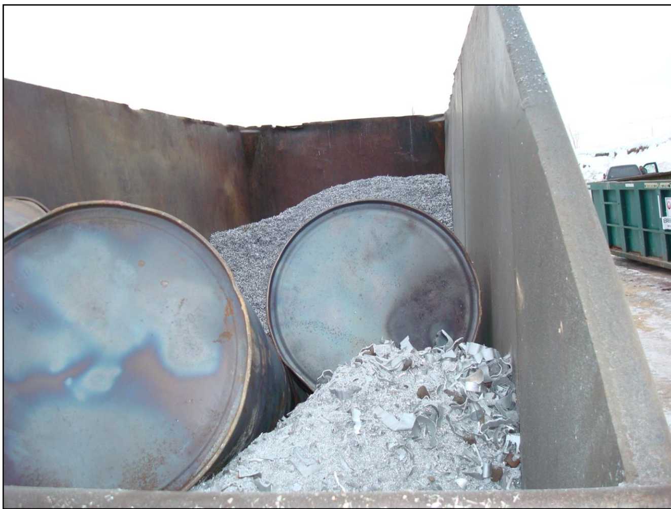
Photo 2. Dumpster contents similar to the contents of the dumpster that exploded. Note thermal pattern and iron oxide (rust) on slag barrels. (NIOSH photo)
