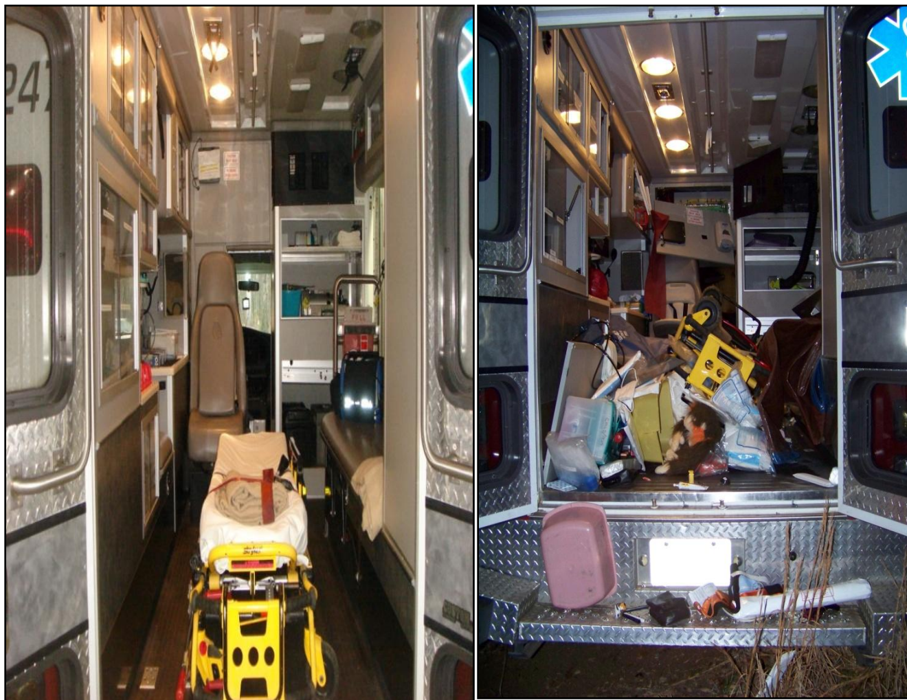
Photos 6 and 7. Typical fire department patient compartment (left photo) and patient compartment of the involved ambulance after the rollover incident (right photo). (NIOSH photo at left, right photo courtesy of fire department.)
