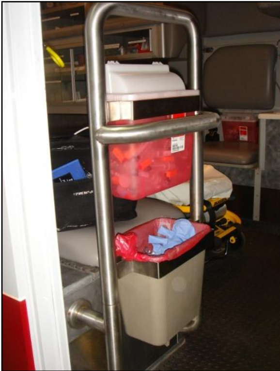
Photos 8 and 9. Typical fire department bench seat support rail (left photo) and bench seat support rail of the involved ambulance after the rollover incident (right photo). (NIOSH photo.)
