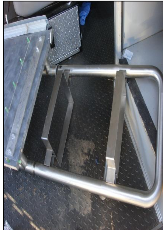
Photos 8 and 9. Typical fire department bench seat support rail (left photo) and bench seat support rail of the involved ambulance after the rollover incident (right photo). (NIOSH photo.)
