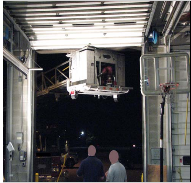
Photos 7 and 8. The photo on the left shows the platform lined up with the damage to the door header. The photo on the right shows the position the platform is believed to have been in when the victim's head got pinned. (Photos courtesy of consultant group.)
