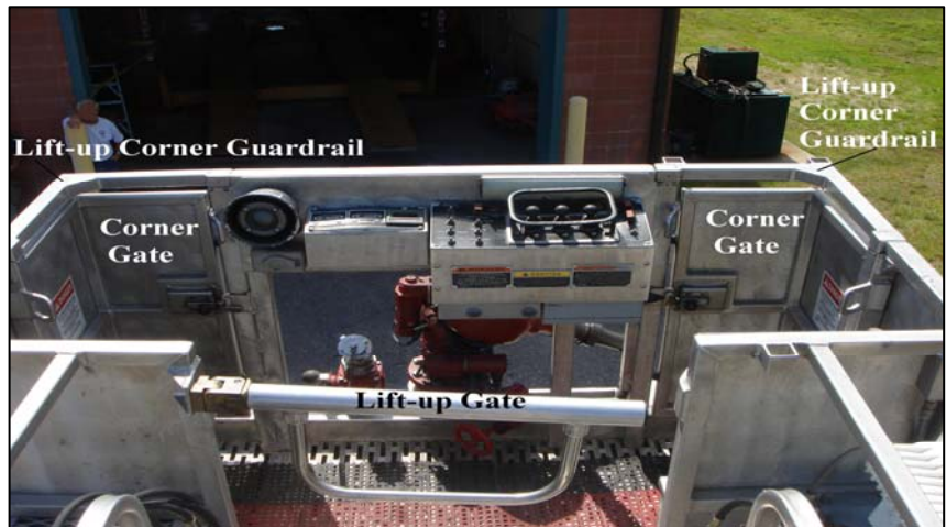
Photo 3. Aerial platform. (NIOSH photo.)
