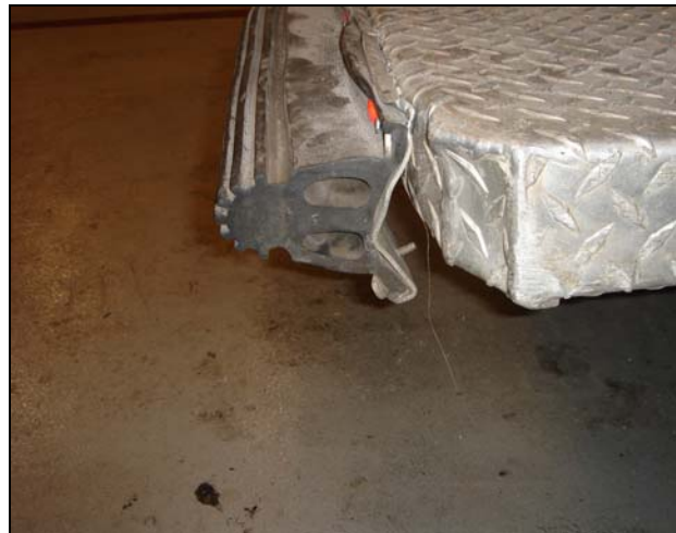
Photos 3 and 4. Pictures show damage to rear bumper and rubber sensor. (Photo courtesy of PEOSH.)
