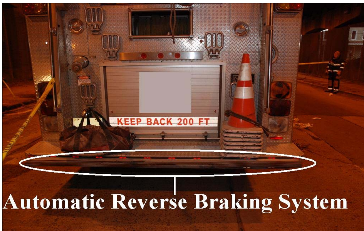
Photo 2. This reverse braking system is attached to the rear bumper of the apparatus and is designed to actuate the rear brakes when pressure is applied to the rubber sensor. (Photo courtesy of sheriff's office.)
