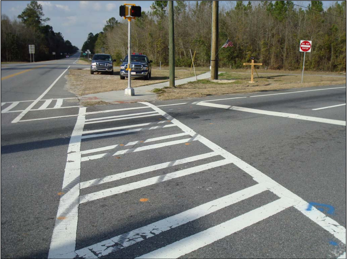
Photo 4. Road markings just before rollover. Note “yaw” marks on roadway. Marks on the right are from the front tires and marks on the left are from the rear tires just prior to the rollover. Tire yaw marks occur when a vehicle slides sideways while still moving forward. In a true yaw, where the vehicle’s rear is attempting to pass the vehicle’s front, each rear tire tracks outside the corresponding front tire. 13
