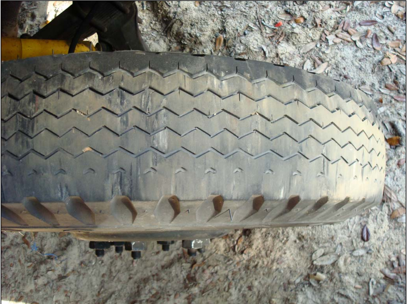
Photo 1. Right front tire tread indicating needed maintenance of steering system and replacement of the tires. (NIOSH photo)
