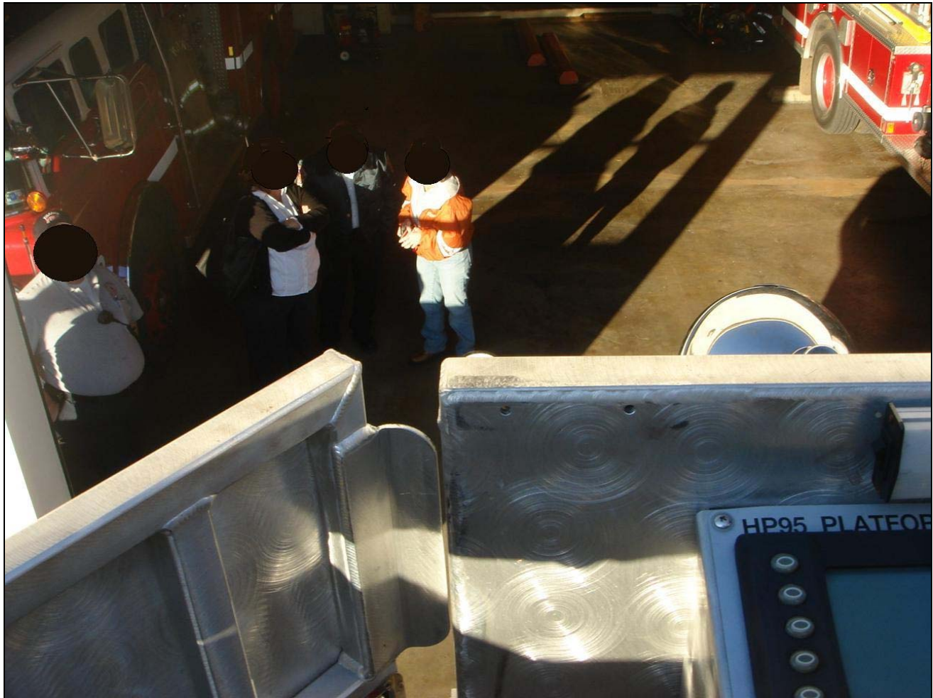
Photo 14. Left platform door. Note door latch and retaining strip designed to keep the door from swinging outward and how door is sprung outward. The door is designed to swing into the platform and when closed, the door is designed to be an integral part of the guard rail system required by NFPA 1901, Chapter 20.7.6.1.2.
