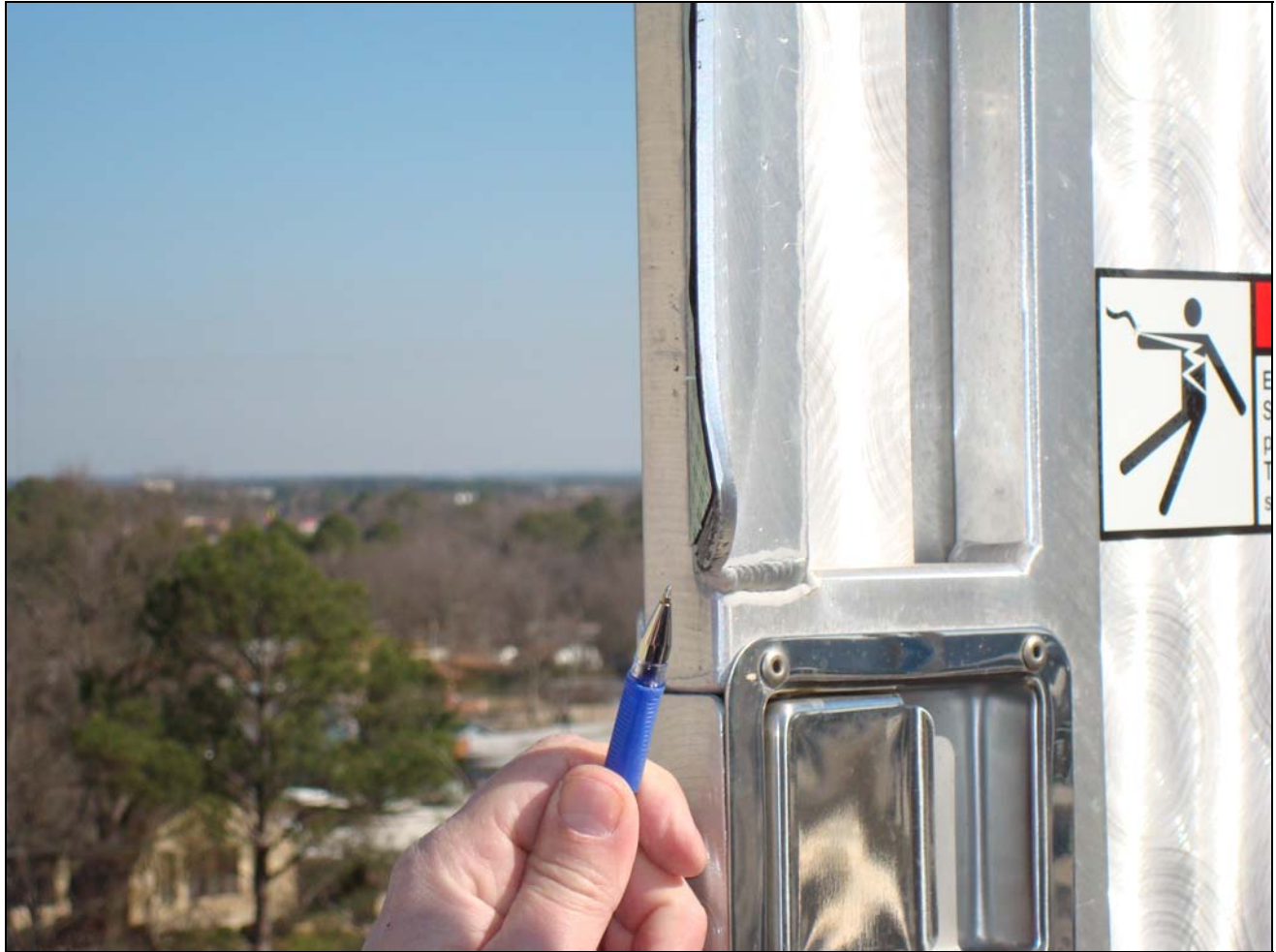
Photo 16. Photo shows the retaining strip on the right platform door is bent inward. One possible cause would be a force applied to the door from within the platform when one of the fire fighters came in contact with the door, causing the door retaining strip to bend inward, allowing the door to open outward.
